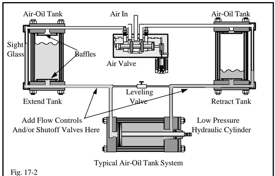
**Tanks, Fig. 17-2.** These tanks hold more than enough oil to stroke the cylinder one way. An **Air Valve** piped to the **Air-Oil Tanks**, forces oil from the tanks into the cylinder. **Add Flow Controls and Shutoff Valves** to the oil lines to give smooth accurate cylinder control.
