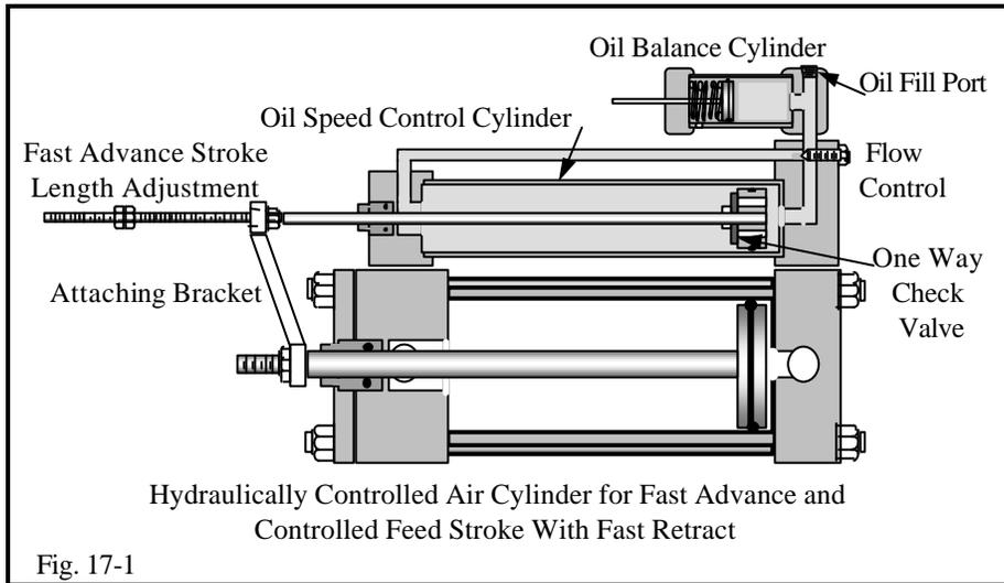
is retarded and controlled by the **Oil Speed Control Cylinder** as oil flows through a **Flow Control**. The air cylinder cannot move any faster than oil flow allows during this part of the cycle. A spring loaded **Oil Balance Cylinder** furnishes oil to makeup for the differential loss from rod to cap. The air cylinder is controlled by oil flow for the remainder of the cycle.
