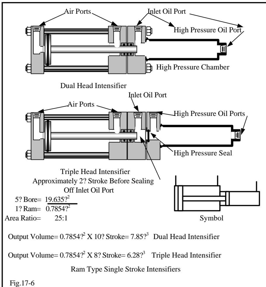
Usually these intensifiers are hydraulic to hydraulic and under a 5:1 ratio. Later there is a similar design for air to air intensifiers up to 4 or 5:1 ratios.
